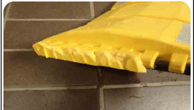
Bad Design, connection pins can not stand small car wheels
